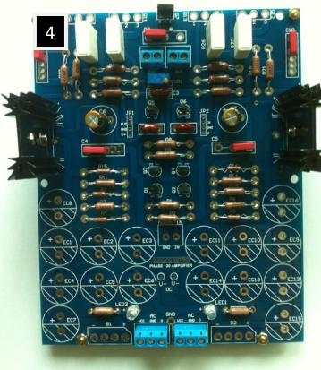
• After completed soldering, connect a DC servo module as shown in below photo (the orange circles). Apply power supply with current limit. e.g. 200mA or fuse. For AC power supply, apply two 20-33V AC to the "AC 0" connectors, where GND is the signal ground that is not connected to the transformer.
