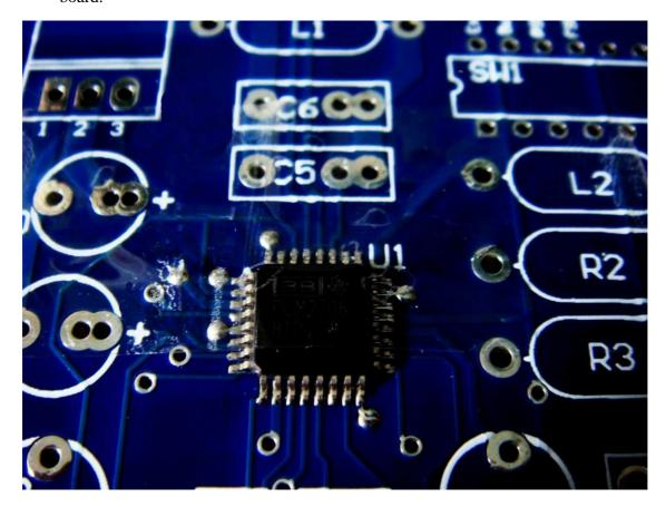
3. Use a soldering iron to heat and then push downward the pin one by one. Avoid heating the pin more than 2-3 seconds which may damage the IC.
