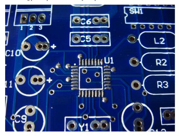
2. Use a plastic tape to mount the PCM2706 IC to the right position. The dot of the IC indicates the direction of the PIN #1. There is a corresponding white dot on the board.
