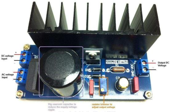
Maximum input-output voltage difference is 29V DC
