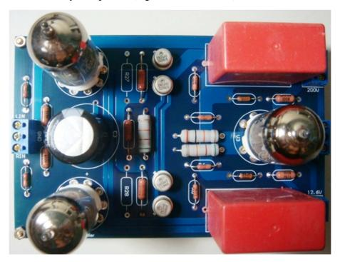
4. Connect the DC power lines 12.6V, +200V, -200V and GND according to the photo.
