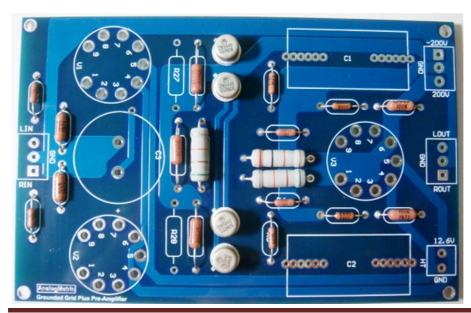
3. Solder the tube sockets, connectors, and then the output capacitors. Note to the polarity of the electrolytic capacitor (big and black in color).
